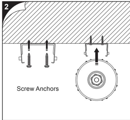
Mount the brackets to ceiling by proper screw anchors and fasteners. Brackets should near end caps
